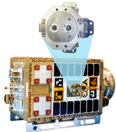
Tanker-001 Tenzing, flown June '21, and closeup of RAFTI Service Valve
